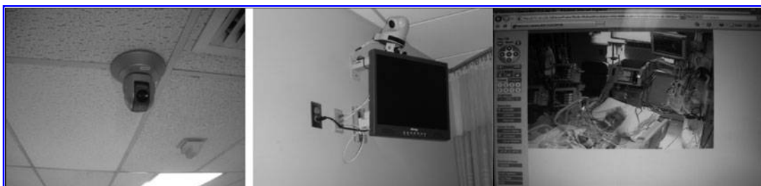
Fig. 6. Simple, fixed cameras located on the ceiling over an ICU bed (left). Sophisticated camera, speaker, and microphone with a screen to show remote Tele-ICU physician (middle). Commercially available software for the remote control of cameras via the Internet (far right).
