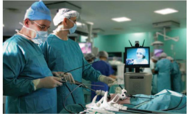
Figure 1. RP6 robot during laparoscopic telerenting.
