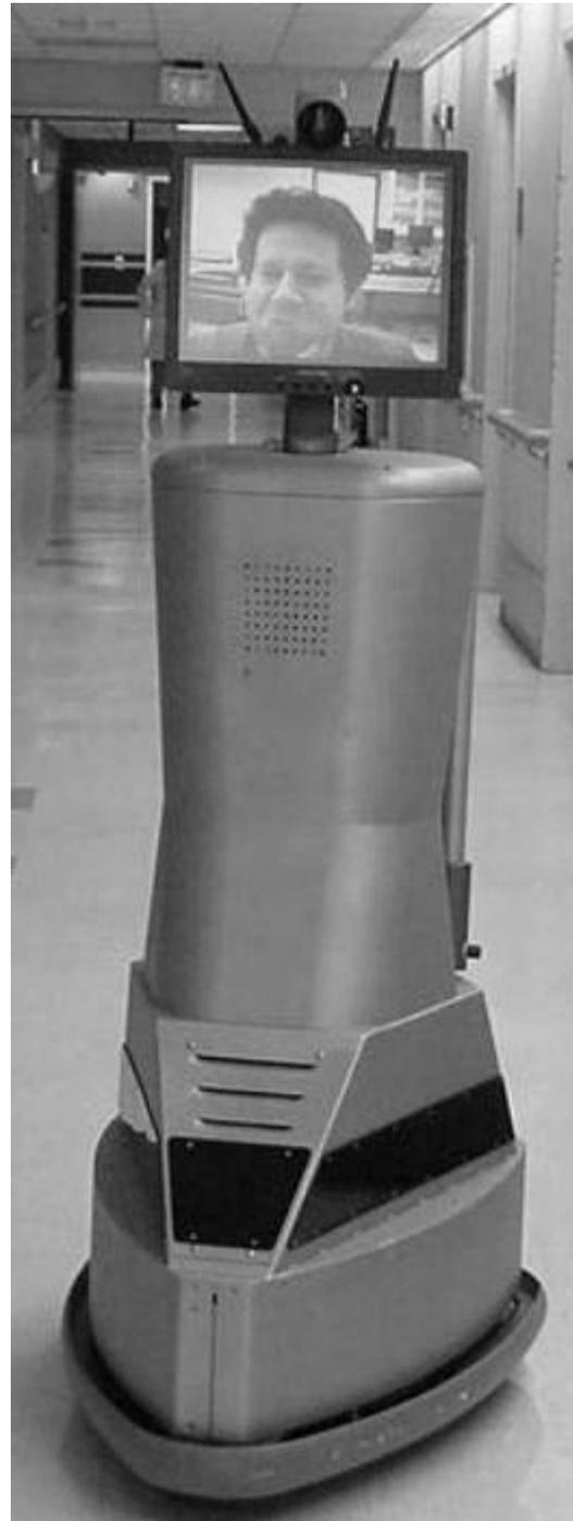
**Figure 1.** The remotely controlled platform of the videoconferencing system carries the camera and the flat-panel monitor with the remote participant's image.
