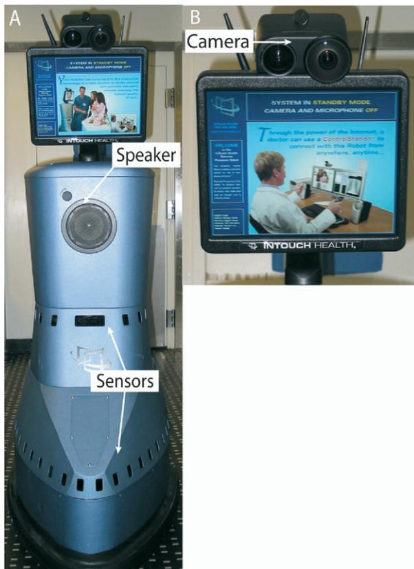
**Figure 1.** (A) Front view of the RP-7 robot demonstrating key components such as speaker, collision avoidance sensors around waist and base, and (B) view of the robot head including the screen, one camera for general purposes such as driving and another camera for zooming, and a microphone.
